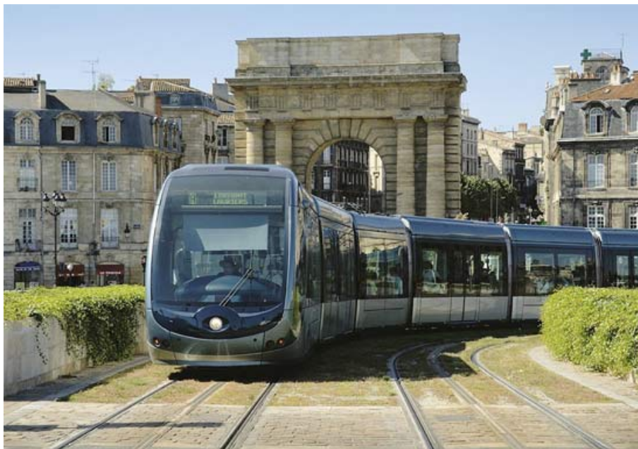
Figure 15: Alstom APS system (here a tram in Bordeaux) which is currently being adapted to heavy trucks (source Alstom).
