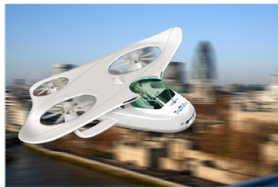
Figure 6: 'Skyrider' - mini airplane PAV (Personal Aerial Vehicle) for individual traffic; EU project mycOpter – Enabling Technologies for Personal Aerial Vehicles; www.mycopter.eu
